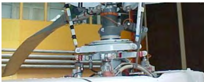
Figure 158 - EC130-B4 Plateau cyclique
