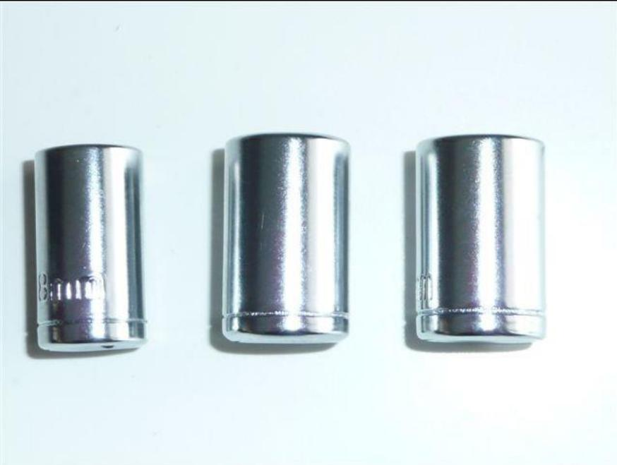
Three silver metal sleeves of different sizes are shown side-by-side on a light blue background. The sleeves are cylindrical and have a slightly textured surface. The leftmost sleeve is the smallest, the middle one is medium-sized, and the rightmost one is the largest. Each sleeve has a small, illegible mark near its base. | 3 douilles n° 8-9-10 | S'utilisent pour serrer ou desserrer diverses fixations sur le vélo. |
