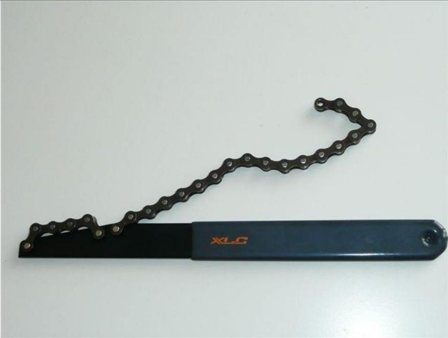
A chain whip tool consisting of a blue handle with the 'XLC' logo in orange, and a black chain attached to the end. The chain is curved upwards. | Fouet à chaîne | S'utilise pour desserrer les pignons ou braquets de la roue arrière.                                   |
