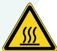
Danger surface chaude
