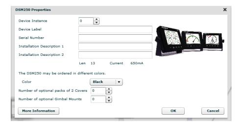
As well as the standard 6 fields for Device Instance, Device Label, Serial Number, Installation Descriptions and the Current Drawn, we also show some options that will affect the Bill of Materials. Change the color to White, and include a Gimbal Mount or extra covers before selecting the OK button.
