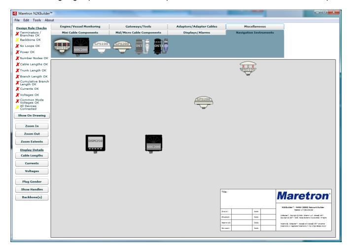
Next add the PowerTap so that we can get power to the network. We are going to use Micro cabling, so choose the Micro/Mid Power Tap Tee from the Mid/Micro Cable Components tab in the Component Library.
