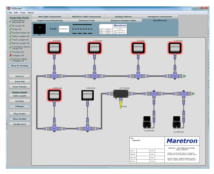
Click the "Show on Drawing" button which will cause some of the DSM250 displays to be highlighted in red. Because of the long cables and high current drain, the voltage drops across the network are too large. We will fix the problem by adding a second PowerTap.
