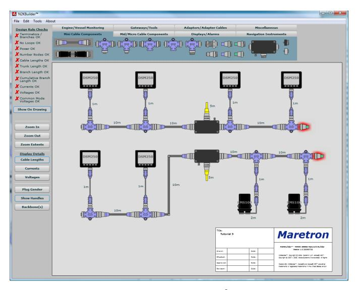
Now connect the last two Tees in the same way. N2KBuilder<sup>®</sup> will detect that both sockets are female, and will use a Field Attachable Cable with two male connectors.
