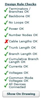
At this point, take a look at the top left of the screen, in the Design Rule Checks Area, to see how compliant our network is to NMEA 2000<sup>®</sup> requirements. We seem to be doing very well.
