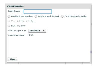
Assume the distance up the mast is 18m. Prebuilt double ended cordsets are limited to 10m, and are therefore not suitable for this design. We need to buy 18m of bulk cable, and then connect a field attachable connector to each end.
