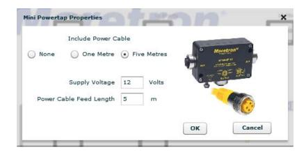
The Power Cable is supplied in one of two lengths, 1m or 5m. The top selection is used to choose which option is included in the BOM.
