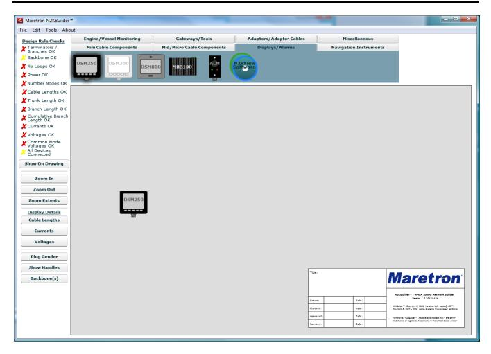
Notice that there is still a DSM250 following the cursor. This enables you drop another component of the same type very quickly without having to go back to the Component Library again. Drop a second DSM250 onto the Drawing Area.
