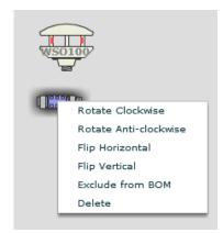
Now we will turn the Micro Inline Termination Resistor around and connect it to the WSO100. Left click on the Micro Inline Termination Resistor to select it, and right click to display the associated menu. The
