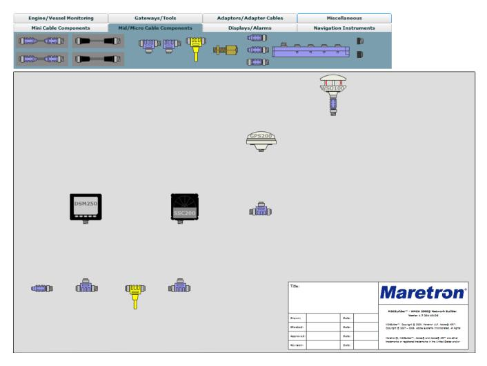
Last, we will add the cables. Micro connectors can have either Micro or Mid size cabling, shown in N2KBuilder® by different thicknesses. Hovering over the cable will also show the thickness. Cables may also be bought with the connectors attached (Double Ended Cordsets) or built from Bulk cable with field attachable connectors.
