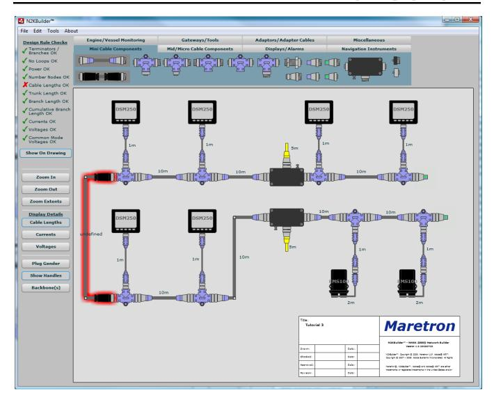
Open the Cable Properties Dialog for the Cable, and set the length to 10m. We also choose to break the Power Cables at both ends of this cable so that the power on each half of the network is isolated from the other half.
