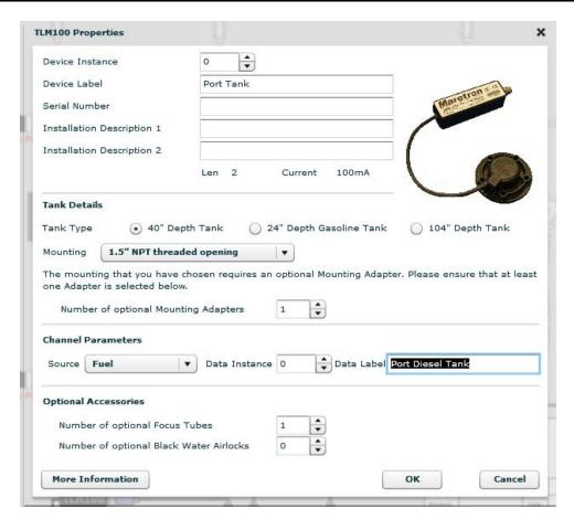
Set up the starboard tank in the same way, with a 1.5" NPT threaded mounting, a Device Label of "Starboard Tank", and a Device Instance of "1". Set the Channel Parameters to "Fuel", the Data Instance to "1" and the Data Label to "Starboard Diesel Tank". We will also order a Focus Tube for the tank.
