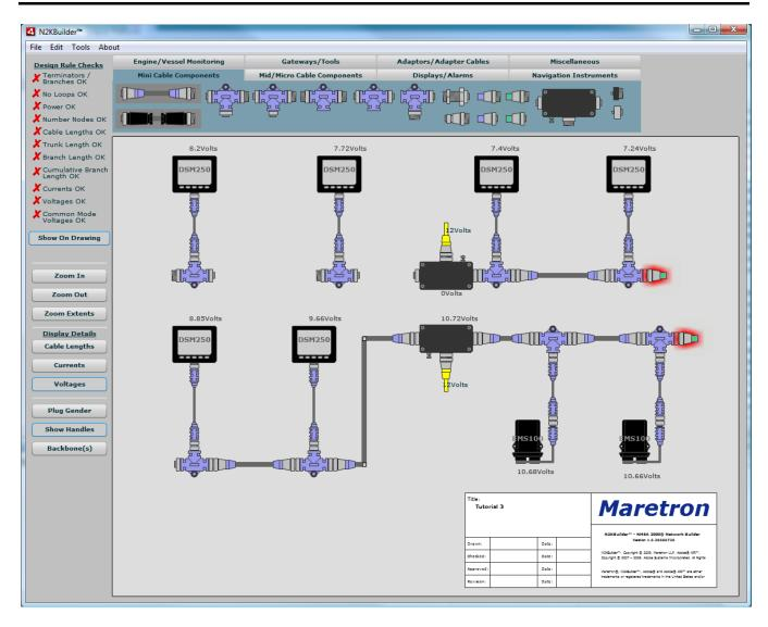
Notice that the female connector from the PowerTap is facing the female connector of the Tee to the left. Flip this Tee and the next Tee horizontally to correctly line up the sockets with the correct genders.
