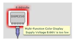
The cables are too thin to supply enough power to the DSM250 at the end of the backbone. This is probably a good time to decide to upgrade the entire network to use Mid cables instead of Micro cables. We could change each cable using the cable Properties Dialog, but there is an easier way using the Network Functions of N2KBuilder<sup>®</sup>. Right click on any cable in the backbone, and select the **Network Functions** option.
