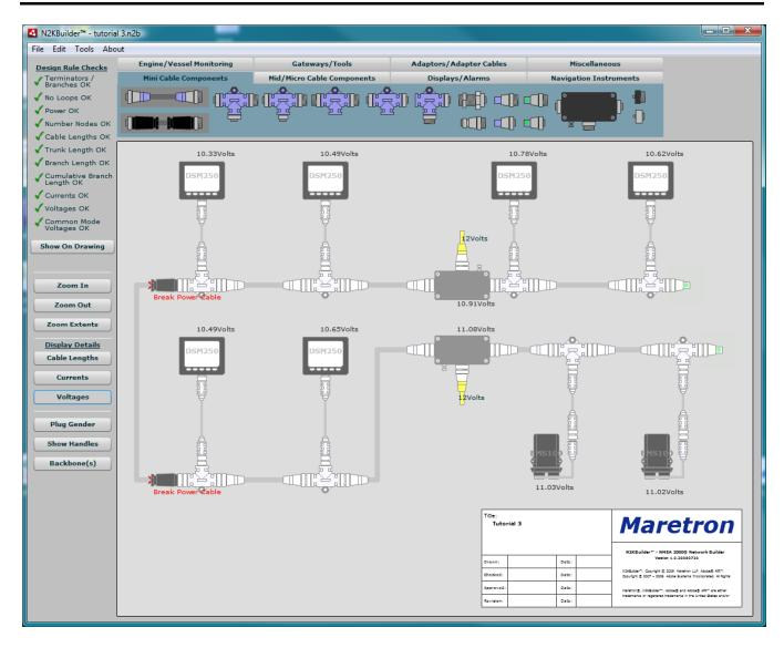
Drag two TLM100 devices and a Multiport Box from the Mid/Micro Cable Components tab. Flip the Multipoint Box horizontally to give the following result.
