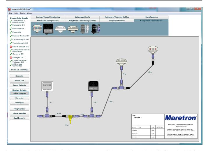
In the **Design Rules Checks Area**, we can see that we now have the **Cable Lengths OK**, but have introduced errors in the Branch Lengths and Voltages. Press the **Show On Drawing** button to highlight the problems.
